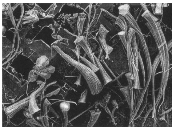
Figure 5. Alien flowers made on an electron microscopy grid from barium sulfate under polymer adsorption control (from the laboratory of M. Antonietti).
